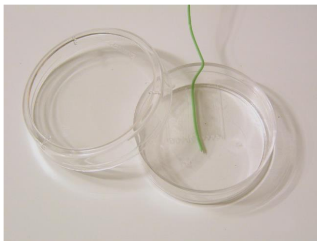
Figure 16. Free Sensor attached on the internal base of the Petri Dish.
