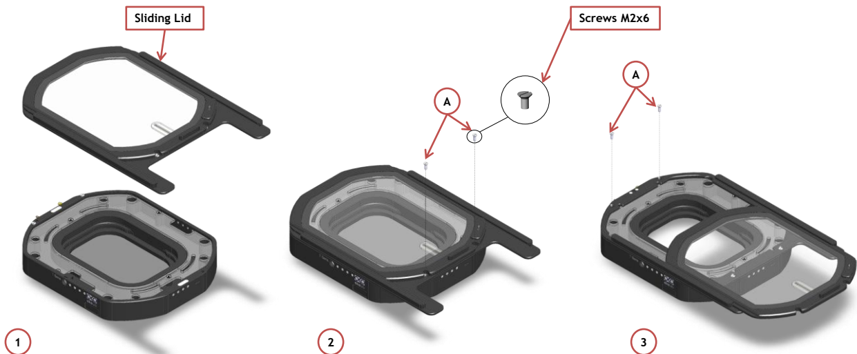
Figure 4. Assembly of the sliding lid
