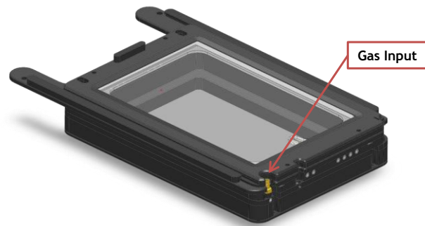
Figure 18. Connection with gas supply.
