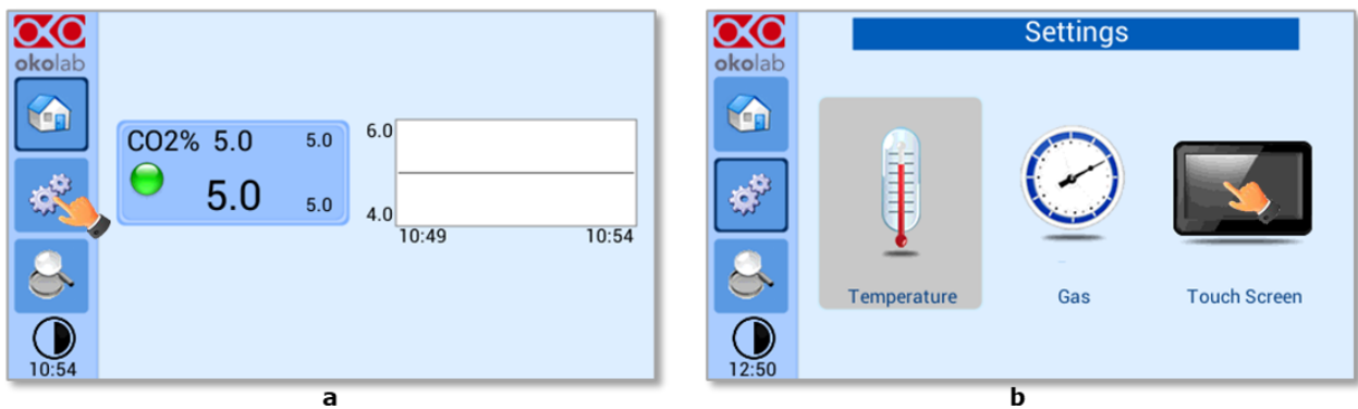
Figure 57 (a) How to enter the setting menu; (b) how to enter the Touch Screen menu.
